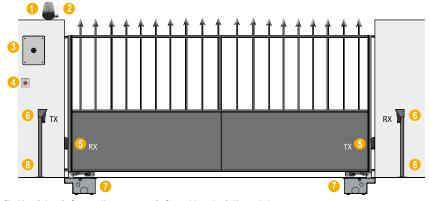
1\_Flashing light 2\_Outstanding antenna 3\_Control board 4\_Key switch
