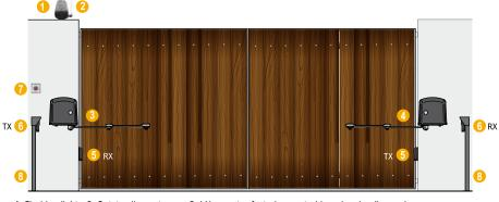
1\_Flashing light 2\_Outstanding antenna 3\_LH operator featuring control board and radio receiver 4\_RH operator 5\_Outer photocell 6\_Inner photocell 7\_Key switch 8\_Photocell posts
