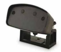
Microwave sensor for vehicle and people detection, suitable for doors and gates. Sensitivity and detection direction can be adjusted separately. Power supply 12-24V dc/ac 2 relay outputs NO/NC - IP67
