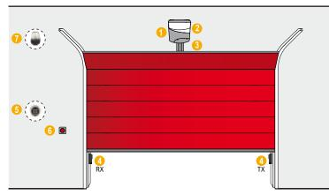
1\_Door opener featuring control board and radio receiver
