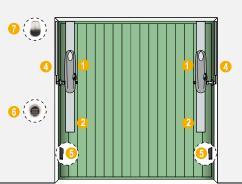
1\_Door opener featuring control board and radio receiver 2\_Drive rack 3\_Fittings for central application 4\_Fittings for side application 5\_Photocells 6\_Wireless keypad 7\_Flashing light
